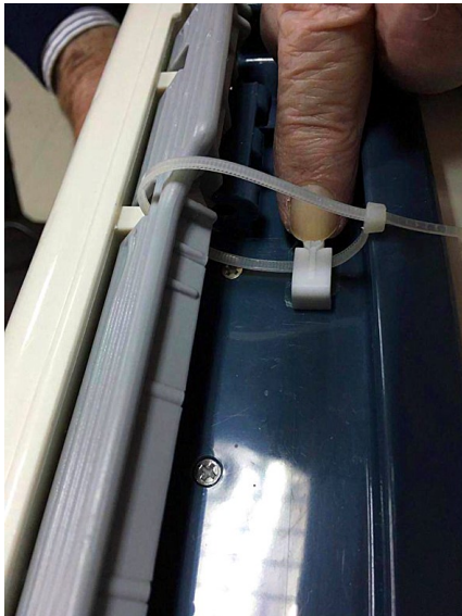
Figure Four – Pass tie through hole in latch
