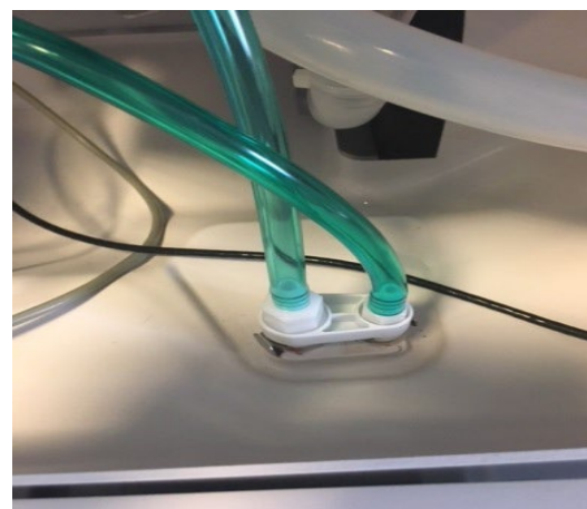
Gas connected to the OCS
